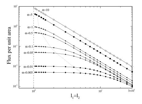
Figure 9: Flux per unit area versus  $l_1 = l_2$  for various values of  $\alpha$  and  $K = \infty$ . The dotted line represents the value of  $l_1 = l_2$  at which the flux per unit area is 90% of its value at  $l_1 = l_2 = 1.05$ .
