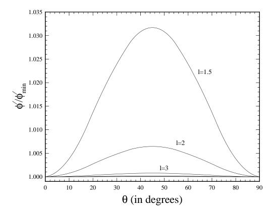
Figure 10: Flux curves divided by their minimums versus  $\theta$  along r = 0.9;  $\alpha = 0.01$ ,  $K = \infty$ , and  $l_1 = l_2 = 1.05, 2, 3, 4, 5, 6$ .
