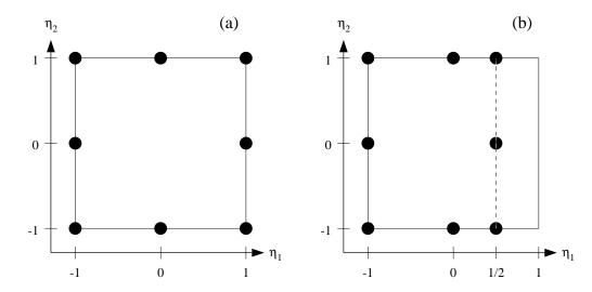
Figure 4: Positions of collocation points for a quadratic element transformed to  $(\eta_1, \eta_2)$  space, (a) normally and (b) when the element is on the edge of the disc, with the nodes positioned to avoid the inverse square root singularity at r = 1.
