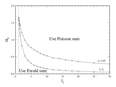
Figure 3: The value of  $\alpha$  at which the Poisson and Ewald summations take the same amount of CPU time versus  $l_2$  for the two cases  $l_1 = l_2$  and  $l_1 = 1.05$ . Above the curves the Poisson sum is more efficient, below the Ewald sum is superior.
