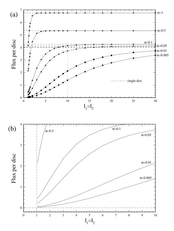
Figure 7: Flux per disc versus  $l_1 = l_2$  for various values of  $\alpha$  and  $K = \infty$ . The graph (b) enlarges the dotted rectangle in (a). The vertical line at  $l_1 = l_2 = 1$  indicates the point at which discs would touch.
