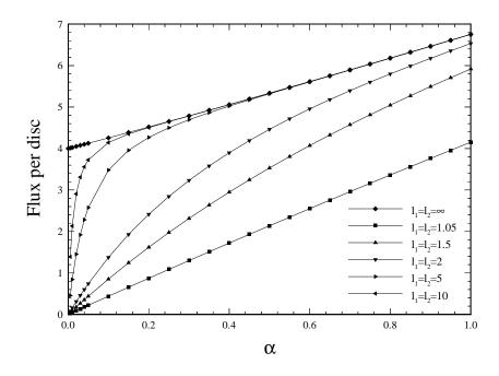
Figure 8: Flux per disc versus  $\alpha$  for various values of  $l_1 = l_2$  and  $K = \infty$ .
