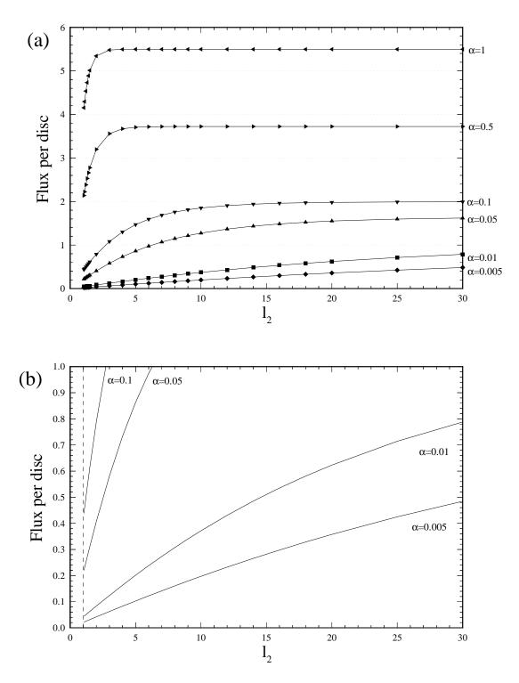
Figure 11: Flux per disc versus  $l_2$  for  $l_1 = 1.05$  and various values of  $\alpha$ . Graph (b) is an expansion of the lower section of (a).
