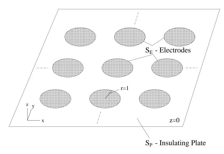
Figure 1: The periodic array of microelectrodes on an insulating plane.
