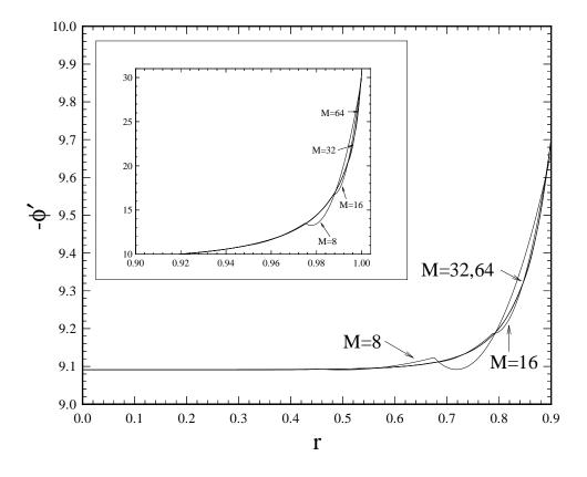
Figure 5:  $-\phi'$  versus r for  $\theta = 0^{\circ}$  for a single microelectrode, varying the number of elements. The parameters are  $\alpha = 10$ , K = 100, and curves are for various numbers of elements in the r direction. The larger graph shows  $-\phi'$  on  $r \in [0, 0.9]$ , with the inset showing the results on  $r \in [0.9, 1]$ . M represents the number of elements in the r direction for the different solutions.
