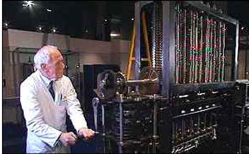
Figure 1: Babbage's Difference Engine No. 2, completed in 1991 for the bicentennial celebration of Babbage's birth, and weighing in at 2.6 tons and 4000 parts, exclusive of the printer, which contains an additional 4000 parts.
