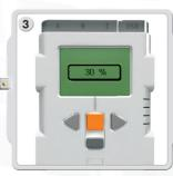
Hold the Light Sensor close to the different colors in your surrounding and see the different readings. You can use the color chart on page 66 of this guide or page 69 of the NXT Building Guide.
