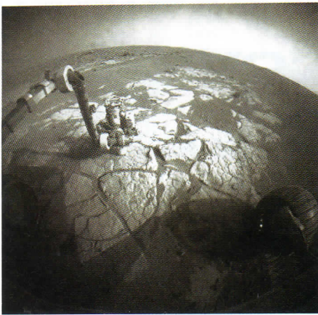
This image taken by the front hazard-avoidance camera on NASA's Mars Exploration Rover Opportunity shows the rover's arm extended to examine the composition of a rock using the alpha particle X-ray spectrometer. Opportunity took this image during the 1,826th Martian day, or sol, of the rover's Mars-surface mission (March 13, 2009).
