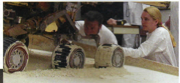
Mike Seibert and Sharon Laubach, engineers on the Mars Exploration Rover team at NASA's Jet Propulsion Laboratory, Pasadena, CA, check the exact position of a test rover in preparation for the next test of a possible maneuver for Spirit to use on Mars. The test setup at JPL simulates a situation in which Spirit is embedded in a patch of soft soil dubbed "Troy," in Mars' Gusev Crater. The July 7, 2009, preparation shown here preceded an assessment of straight-backward driving the next day—one of several possible maneuvers to be assessed in the test sandbox before further driving commands will be sent to Spirit.
